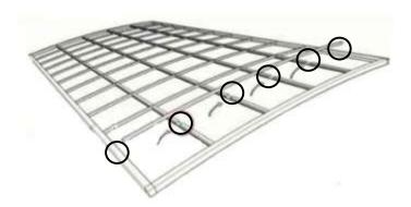
• Lift roof frame up on to the Roof Beams. Secure roof frame to beams with screw #4. There are 12 intersection points, Secure with 4 x screw #4 per intersection circled and 2 x screw #4 per intersection marked with a square.
