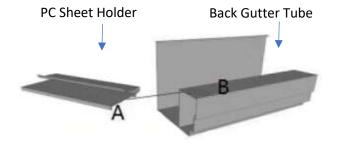
A groove should slot into B plate
