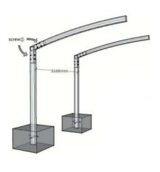
**Step 3: Roof Frame Construction**
